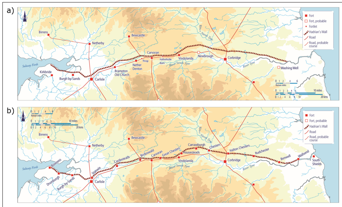
Figure 3: The changing design of the Hadrian's Wall (a) as originally conceived and (b) following the 'fort decision'. Changes included the addition of forts along the line of the curtain and a switch to construction entirely of stone, as opposed to the earlier use of turf in the western sector (CC BY-NC 3.0; Courtesy of David Breeze, reproduced with permission).
