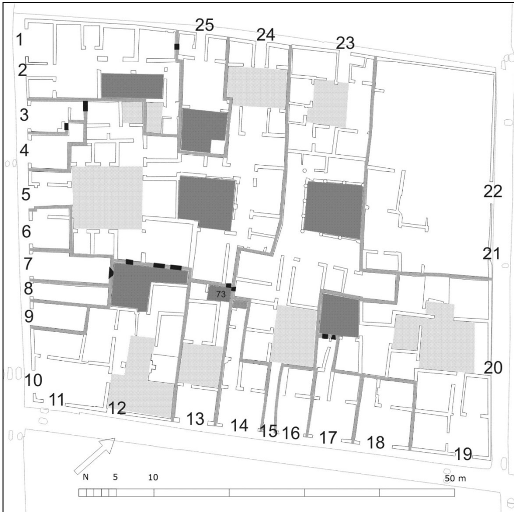
Figure 3: The distribution of windows (in black) between houses in Insula IX.3. Roofless spaces onto which these windows opened are shaded dark grey, and partly unroofed spaces are shown in light grey (EPUH/M. Holappa/H. Ynnilä).
