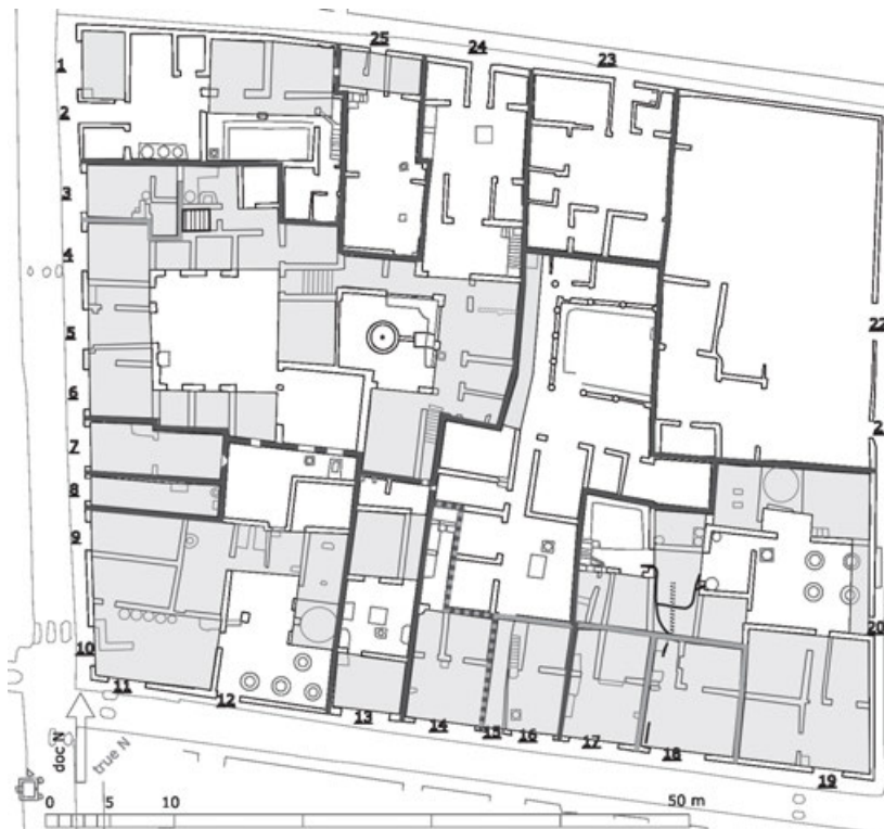
Figure 3: Shared structures between units in insula IX.3. Windows piercing walls between units are in white, a shared cess pool between Units IX.3.3 and 5/24 is striped, a shared water pipe between Units IX.3.18 and 19–20 is shown as a black line and a drain shared by them is marked with broken black lines. The extension of upper floors in each unit is indicated in light grey and the borders of units on upper floor level are indicated in mid-grey (compare Fig. 2 showing the borders of units on ground floor level). Unit clusters indicating common ownership are bordered in dark grey. The common ownership of Units IX.3.14 and 15 is not clear which is indicated with a broken line. Plan: EPUH/M. Holappa, H. Ynnilä
